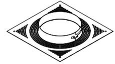
1. Frame a four sided level square opening within the joists using timber stringers where necessary to allow for the correct distance to combustibles from the outer wall of the chimney. This distance must be a minimum of 60mm for solid fuel applications.
