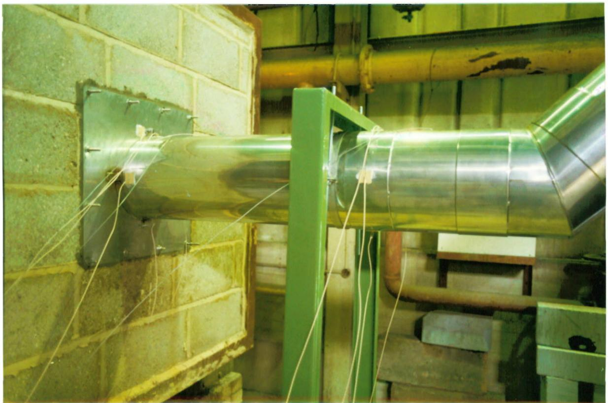
Plate 5 Chimney and penetration seal outside furnace before test
