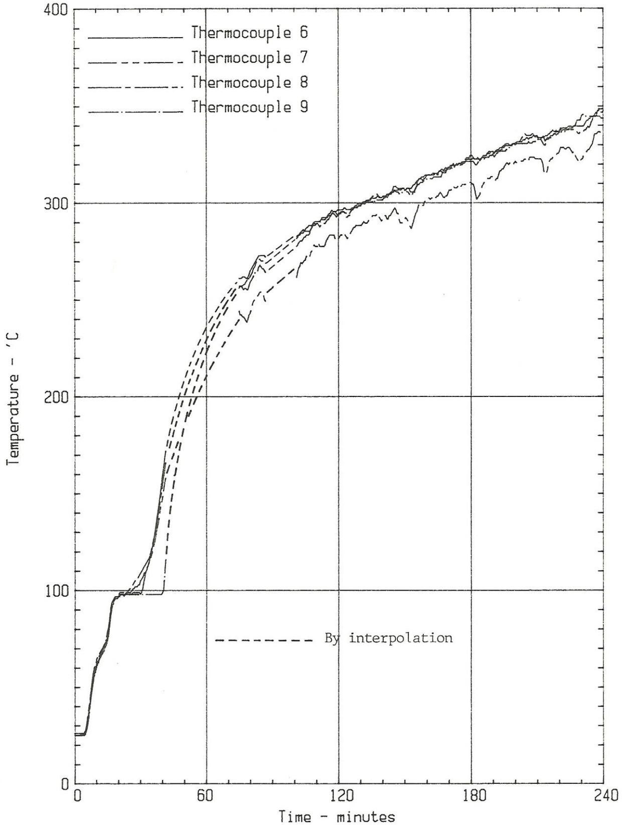
Figure 5 - Temperatures on outer surfaces
