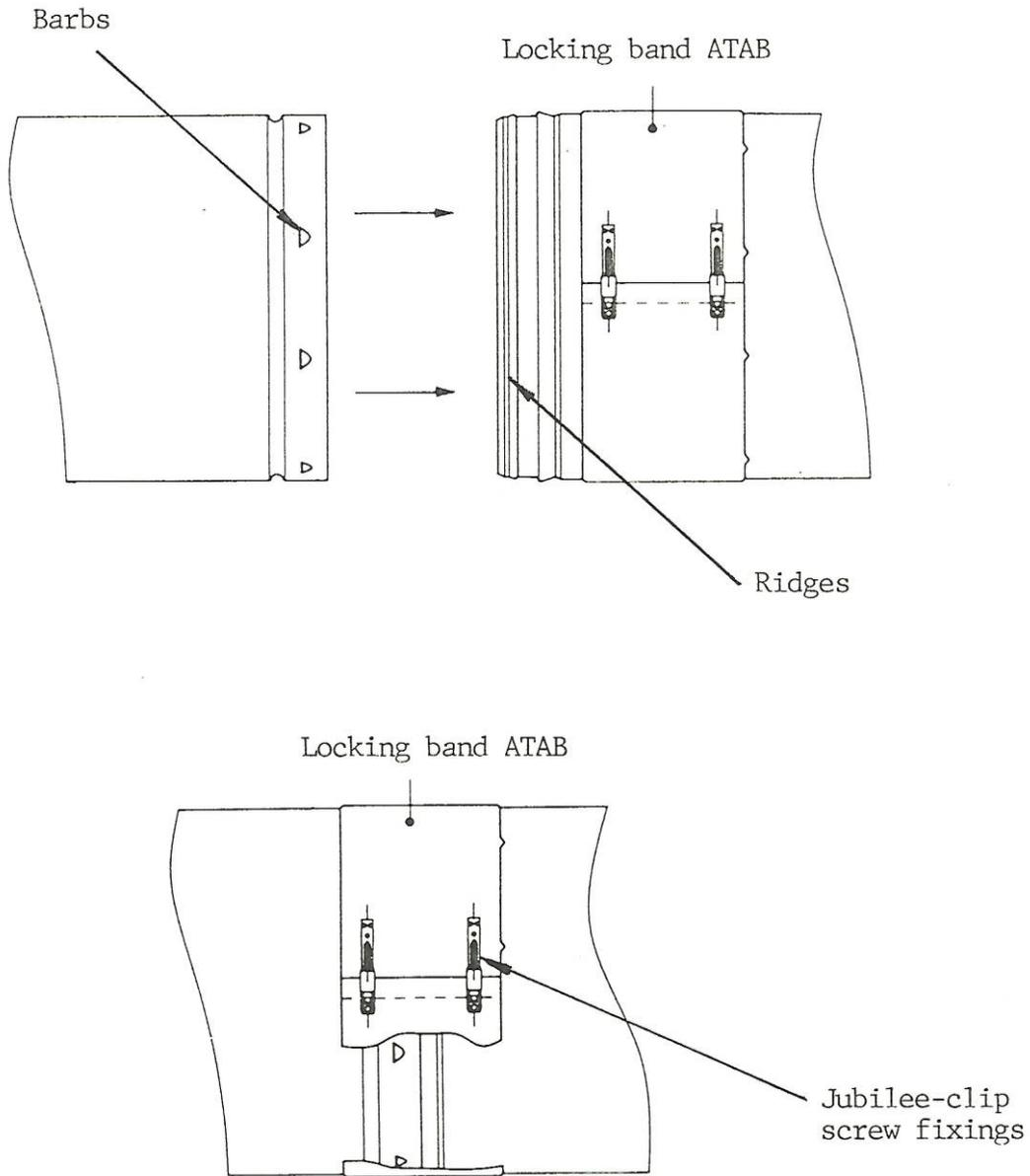
Figure 2 Jointing system for Metaloterm AT chimney sections
