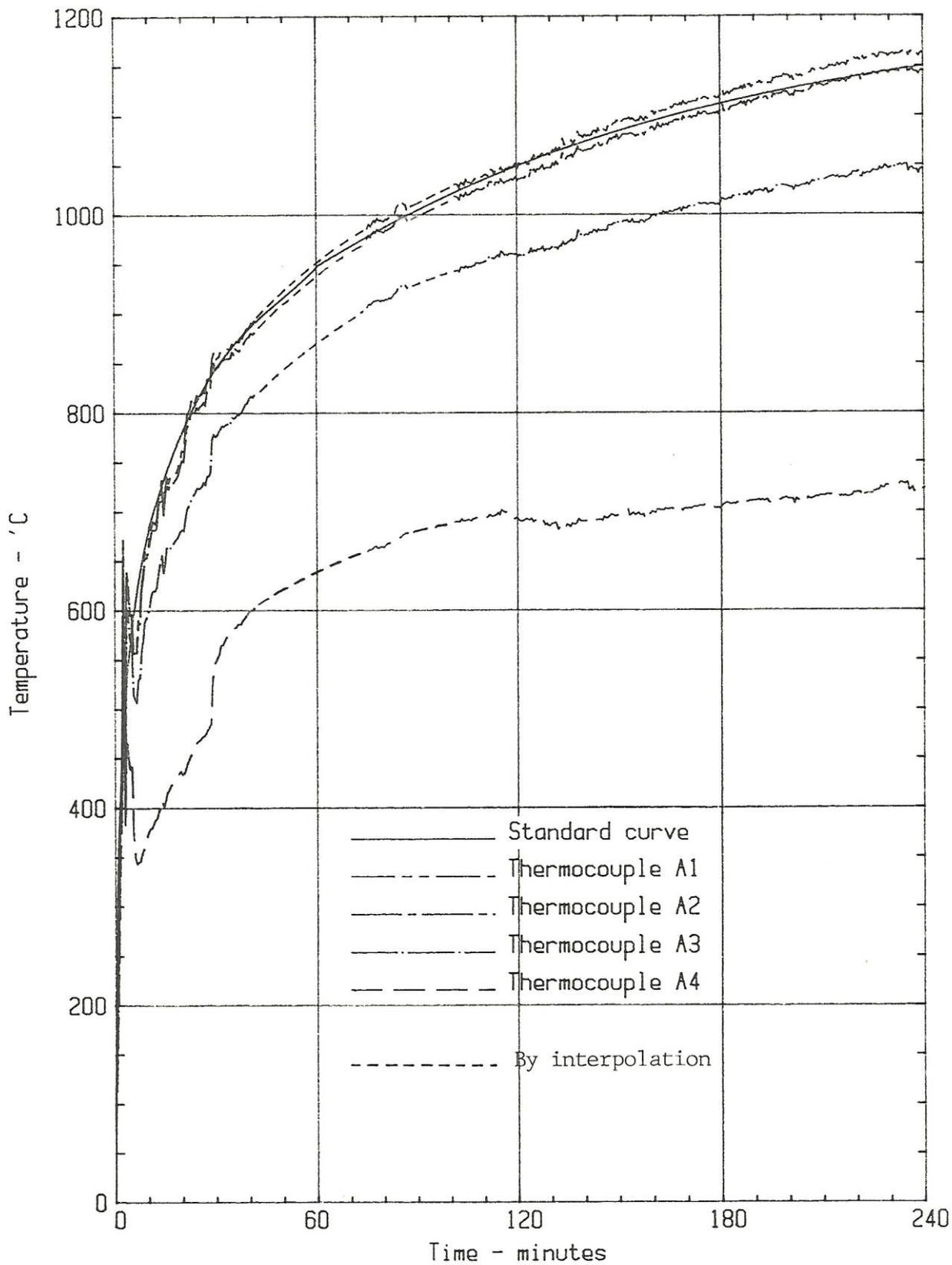
Figure 3 - Temperatures inside flue
