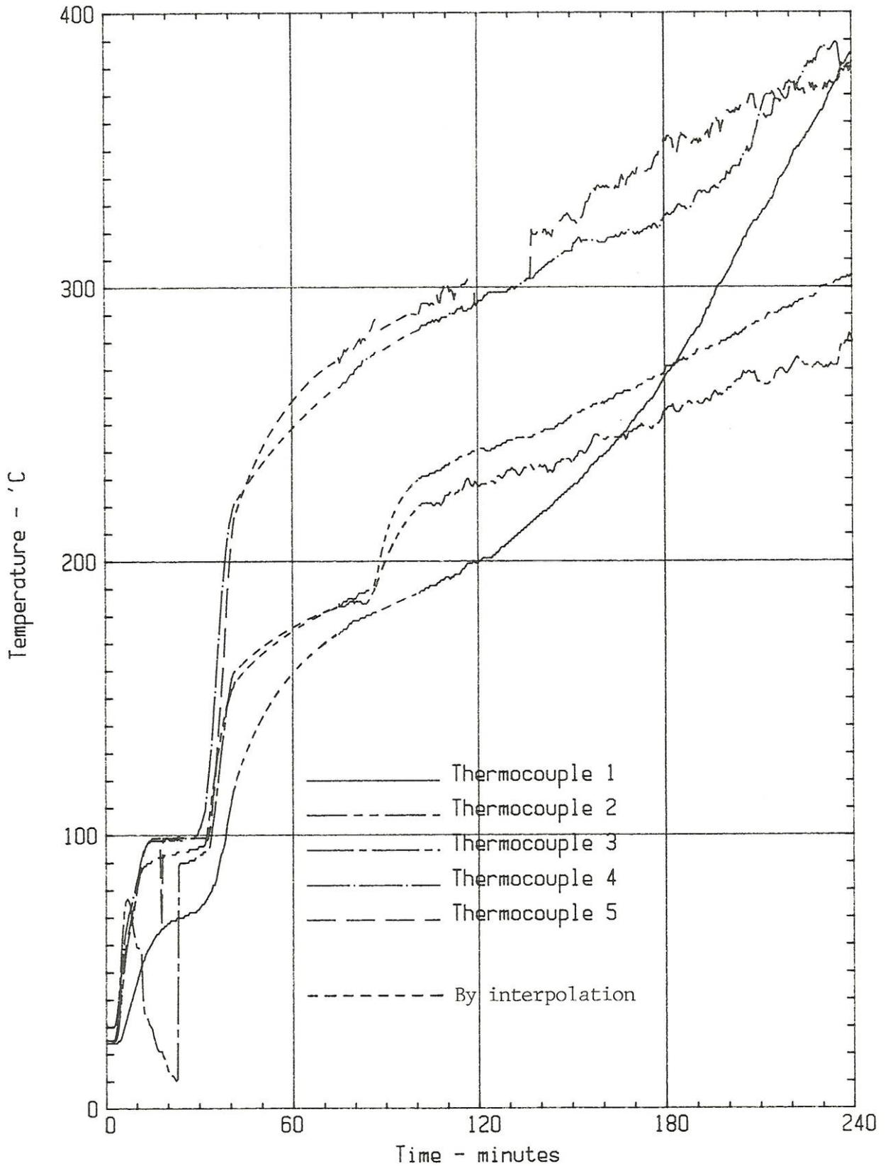
Figure 4 - Temperatures on outer surfaces
