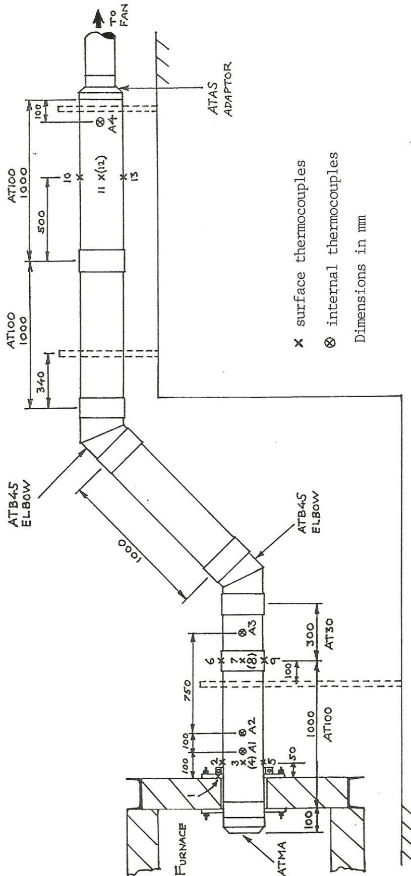
Figure 1 Arrangement of chimney sections and thermocouple positions
