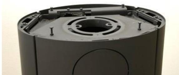
1.) Remove the top plate and take off the outer air inlet and inner flue tube supports.
