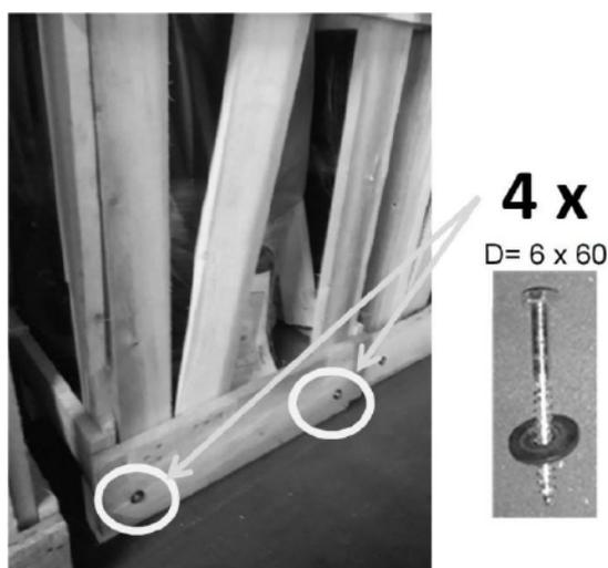
To remove the wooden crate, four screws have to be removed (one on each corner).
