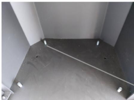
Adjusting screws for uneven floor (4x)
