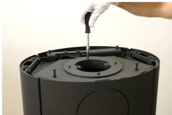
2.) Stick the seal for the central supply air feed (accessory component 2) onto the inner and outer edge of the cover for the upper central supply air feed (accessory component 7) and attach it to the stove.
