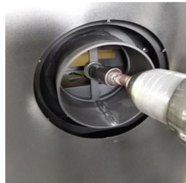
2.) Unscrew the M8 bolt in the inner combustion air panel and remove the panel
