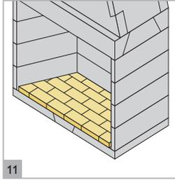
11 Cut 50mm thick fire-bricks and lay loose on the base. Glue the front row of bricks with fire-brick mortar as per the instructions on the bag.
