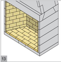
13 Cut 25mm thick fire-bricks and glue to the sides of firechest with fire-brick mortar.
