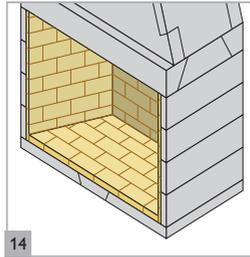
14 Point in the fire-bricks with the fire-brick mortar and wipe away excess.
