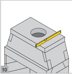
10 Bed on the top plate slab. Check all plumb and level, remove any excess glue.
