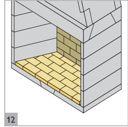
12 Cut 50mm thick fire-bricks and glue to the back of firechest with fire-brick mortar.
