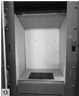
The door is removed first (the door can be lifted off at approx. 10 cm open position).
