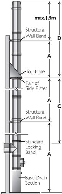
**Wall Mounted Installation with pair of Cantilever Brackets and Structural Locking Bands**
