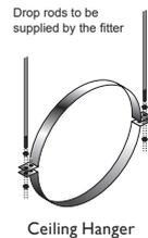
1. Position the split band around the chimney section and fasten using the nuts and bolts provided. The second bolt hole on the arms of the band is to allow for connection of the screwed rod, which will be provided by the installer.
