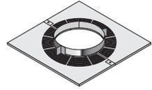
1. Frame a four sided level square opening within the joists using timber stringers where necessary to allow for the correct distance to combustibles from the outer wall of the chimney. This distance must be a minimum of 50mm on Gas and Oil applications and 60mm for solid fuel applications (see Fig. 3 below - distance x).
