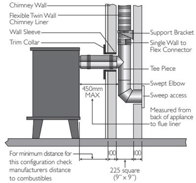
**Top Outlet Twin Wall Connecting Flue Pipe into Re-lined Masonry Chimney**
