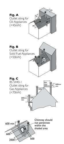
1. The weather surface is the building external surface, such as its roof, tiles or external walls.
