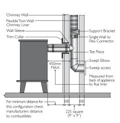
Rear Outlet Twin Wall Connecting Flue Pipe into Re-lined Masonry Chimney
