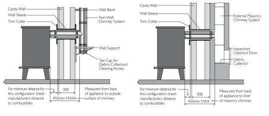
Rear Outlet Twin Wall Connecting Flue Pipe Through Cavity Wall into Twin Wall System Chimney
